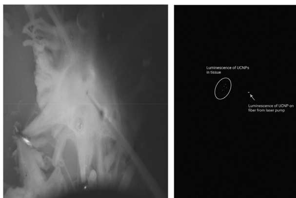
Fig. 1. Snail nervous system microphotography with optical fiber (left) and upconversion nanoparticles in the tissue illuminated by 980 nm laser through fiber (right).
